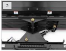
1. 4° SIDE-TO-SIDE OSCILLATION FOLLOWS UNEVEN SURFACES
