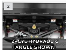
1. 4" SIDE-TO-SIDE OSCILLATION FOLLOWS UNEVEN SURFACES
