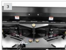
1. 4' SIDE-TO-SIDE OSCILLATION FOLLOWS UNEVEN SURFACES
